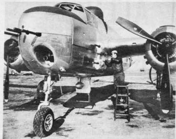
"Flying 75" is augmented by four machine guns in nose and two package guns mounted on either side.
